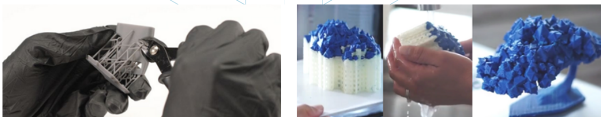
Figure 8: Mechanical process and bath for removing the support structures. [17] [18]
